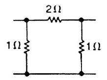
b) Find driving point admittance function for the given one port network.
